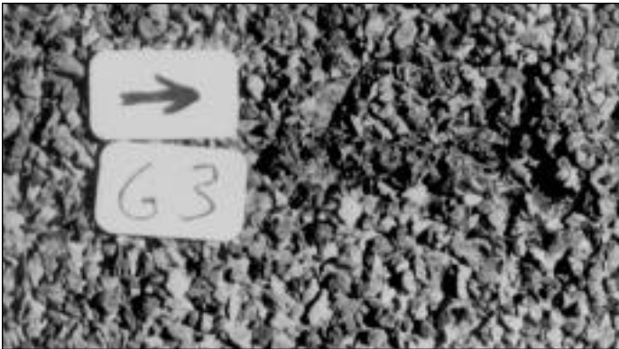
Photo 8. Close-up of Tab G-3, half-panel designation CO-FS-D-0 at 10 years 6 months weathering exposure. Note impact-caused fracture.
